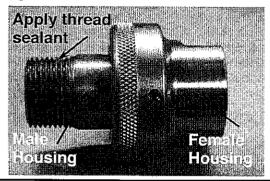
Step 3: Apply Teflon tape or other thread sealant to the 1"
