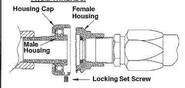
**Step 5:** Remove the Seal and O-Ring from the Female Housing.
