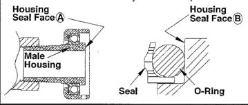
**Step 7:** Lightly lubricate the replacement O-Ring <u>only</u> with Dow 111 lubricant (provided when Seal Kit is ordered).
