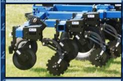
BLU-JET MaxPac Spring Bundles ensure accurate depth in heavy soil types with rocks
