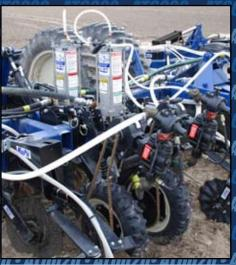
Double GDI Precision Ammonia Metering Systems for high rate, high speed, cold weather operation
