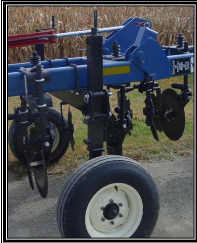
In the inline transport position showing screw type transport wheels, wing lockup with tow tongue attached
