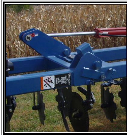
In the inline transport position showing screw type transport wheels, wing lockup with tow tongue attached
