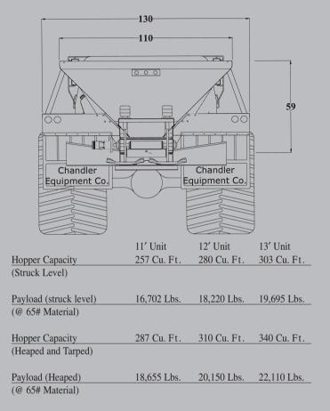
All Products and Specifications subject to change without notice. Drawing shown with 45 degree slope sides and 24" Belt Over Bar Chain.
